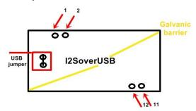
Pin 1 have to be tied to pin 12 and pin 2 (GND) have to be tied to pin 11 (GND).
