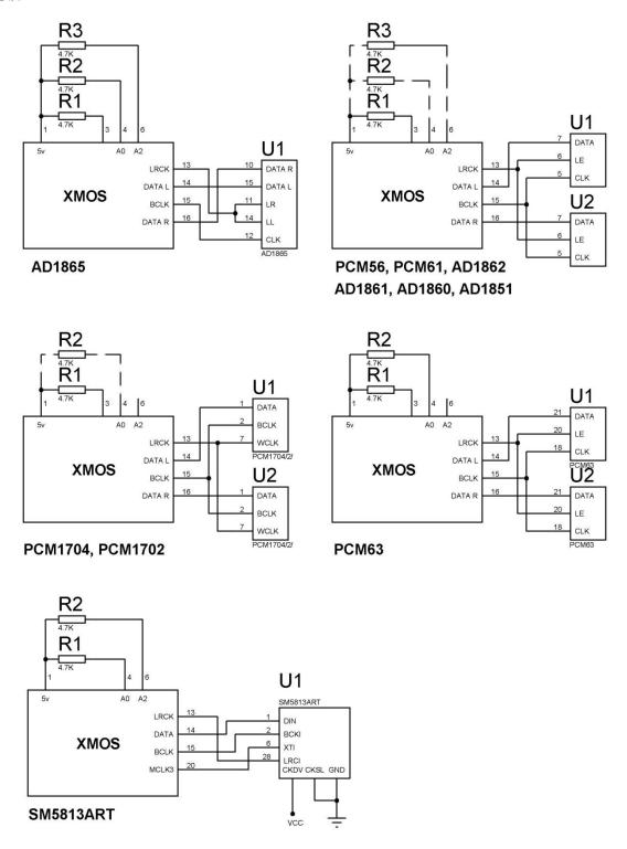
Note: One have to connect the GND (pin11) of the I2SoverUSB board to the Digital GND of the used DAC.
