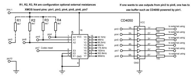
A0, A1 and A2 outputs could be load with CMOS input level (3.3V).
