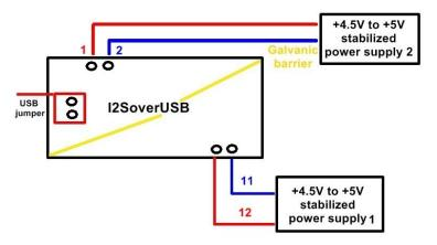
The computer recognizes the boards only if all power supplies are provided (all three ways to power the board), no matter the order of providing power supplies.
