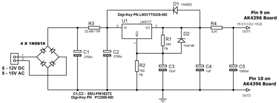
External power supply for AK4396 and generators and reclocks on I2SoverUSB board.
